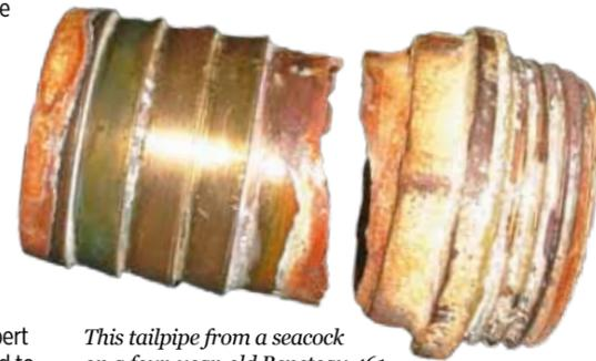
This tailpipe from a seacock on a four-year-old Beneteau 461 sheared off at the inboard end
