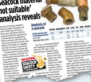
AUGUST 2011 YM sent a failed seacock from a three-year-old Hanse 470e for analysis. Severe electrolytic corrosion caused a through-hull fitting to fall off the outside of the hull of his 40ft ketch
