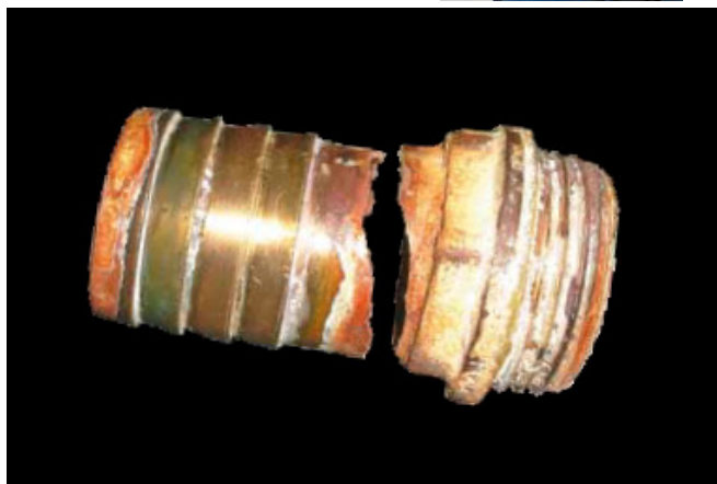
This tailpipe from a seacock on a four-year-old Beneteau 461 sheared off at the inboard end
