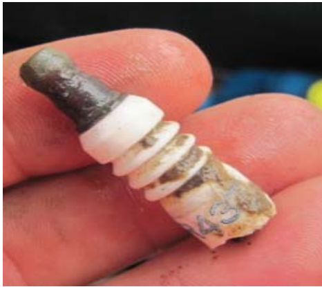
Broken spark plug
